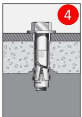
Tighten DynaBolt™ Plus Anchor Hex Bolt
