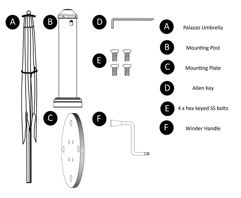
The Palazzo is best mounted onto a 100mm reinforced concrete slab with 4 x 10mm x 105mm Stainless steel bolts. These need to be purchased separately (not supplied).
