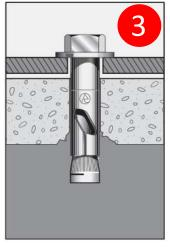
After mounting the rotate bearing to the onground plate Insert DynaBolt™ Plus Anchor Hex Bolt through the onground plate and tap lightly with hammer until washer contacts fixture.
