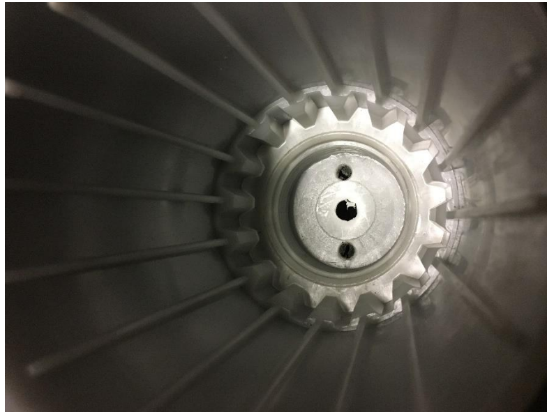
Internal Locking Assembly of base – Note notches
